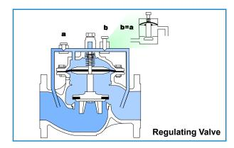
The 2-way control device provides sensitive, accurate, and constant modulating, control of the main valve. The main valve does not fully open, as the control device prevents total draining of the control chamber. The 2-way control device is standard in most pressure regulating valves.
