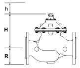
$h^{\star}$  = minimal required maintenance space End Connections (for PN16 or PN25) ISO 2084, 2441, 5752 ANSI B16, AS2129, JIS B22.
