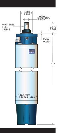
Note: 60 Hz - 3,450 RPM. 50 Hz - 2,875 RPM
