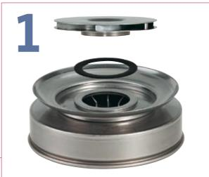
Loss of efficiency has been reduced to an absolute minimum in the impeller stack of the Grundfos CR pumps. This has been achieved for instance by applying a floating seal ring as a perfect seal between the individual chambers.
