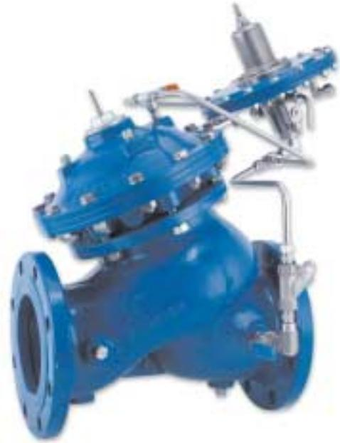
The Model 750-80-X Level Control Valve is a hydraulically-controlled, diaphragm-actuated, control valve that shuts-off at pre-set reservoir high-level and fully opens in response to an approximately one-meter (three-foot) level drop, as sensed by the 3-way altitude pilot mounted on the main valve.
