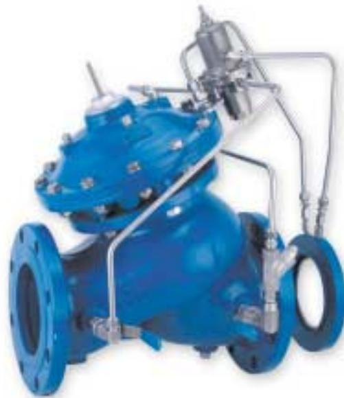
The Model 770-U Flow Control Valve is a hydraulically-operated, diaphragm-actuated, control valve that maintains pre-set maximum flow, regardless of fluctuating demand or varying system pressure.
