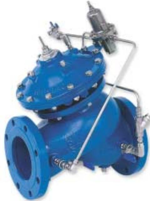
The Model 720 Pressure-Reducing Valve is a hydraulically-operated, diaphragm-actuated, control valve that reduces higher upstream pressure to lower constant downstream pressure regardless of fluctuating demand or varying upstream pressure.
