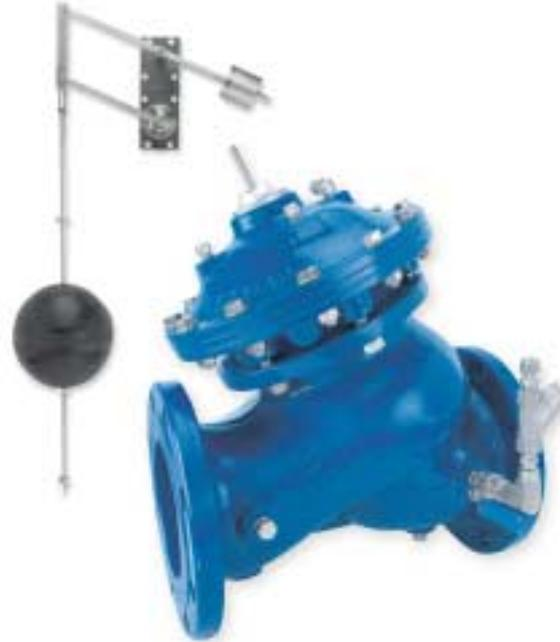
The Model 750-66-B Level Control Valve with Bi-Level Vertical Float is a hydraulically-controlled, diaphragm-actuated, double-chambered control valve. The valve is hydraulically powered to fully open at pre-set reservoir low-level, and to shut-off at pre-set high level regardless of valve differential pressure.
