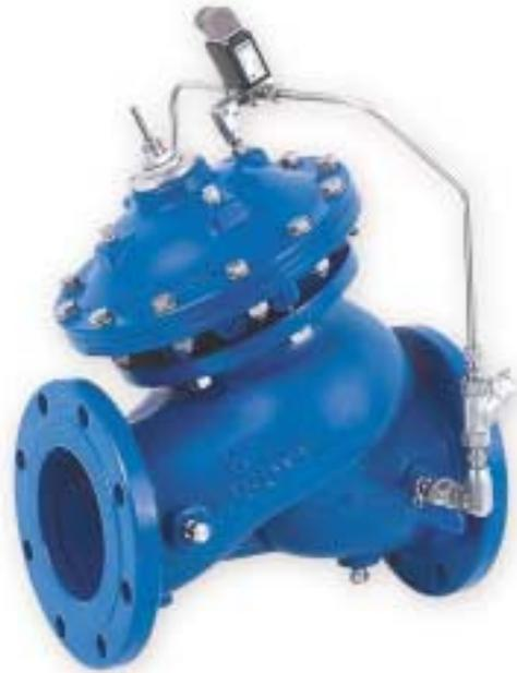
The Model 710 Solenoid-Controlled Valve is a hydraulically-operated, diaphragm-actuated, control valve that either opens fully or shuts-off in response to electric signals. For very low-pressure applications, refer to the Full-powered Opening & Closing Model 710-B.
