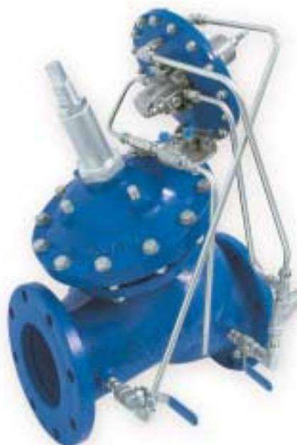
The Model 790-M Burst Control Valve is a hydraulically-operated, diaphragm-actuated, control valve that upon sensing flow in excess of setting shuts-off and locks drip-tight, until it is manually reset. As long as flow is lower than the setting, the valve remains fully open, minimizing head-loss.
