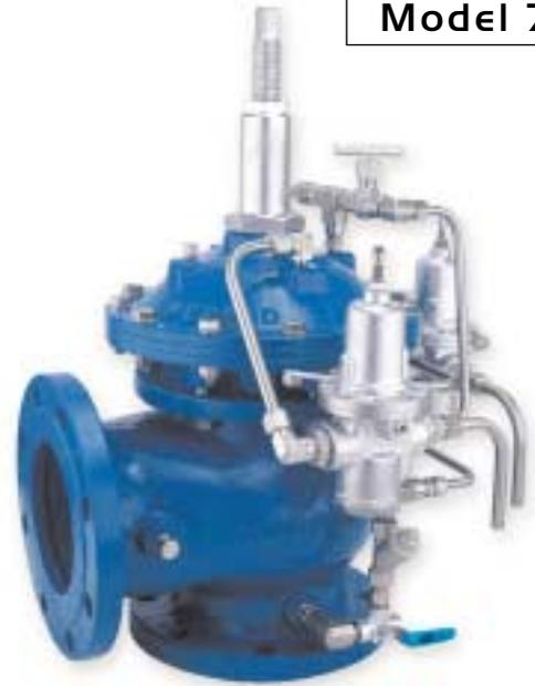
The Model 735-M Surge-Anticipating Valve is an off-line, hydraulically-operated, diaphragm-actuated valve. The valve, sensing line pressure, opens in response to the pressure drop associated with abrupt pump stoppage. The pre-opened valve dissipates the returning high pressure wave, eliminating the surge.
