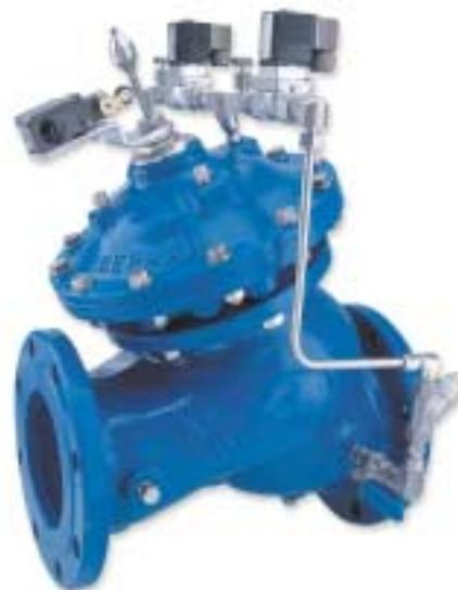
The Model 718-03 Electronic-Control Valve combines the advantages of an excellent modulating, line-pressure driven, hydraulic control valve with the advantages of electronic control. This valve responds to signals from the (optional) BERMAD BE electronic controller according to the set values programmed into the controller.
