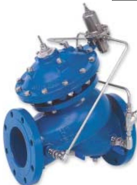
The Model 730 Pressure-Relief/Sustaining Valve is a hydraulically-operated, diaphragm-actuated, control valve that can fulfill either of two separate functions. When installed in-line, it sustains minimum pre-set, upstream (back-) pressure regardless of fluctuating flow or varying downstream pressure. When installed as a circulation valve, it relieves excessive line-pressure when above maximum pre-set.
