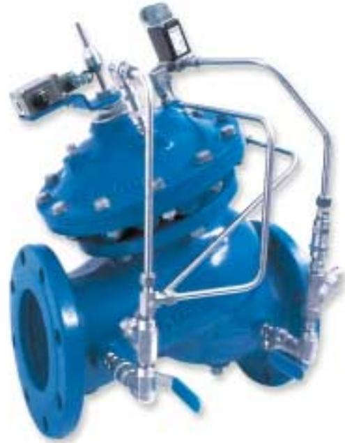
The Model 740 Booster-Pump Control Valve is a hydraulically-operated, diaphragm-actuated, active check valve that opens fully or shuts off in response to electric signals. It isolates the pump from the system during pump starting and stopping, to prevent pipeline surges.
