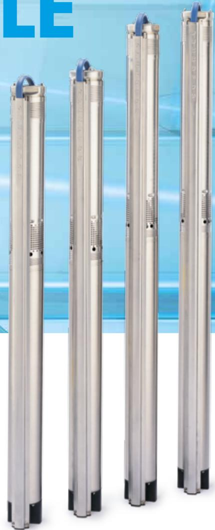
The SQ pump is Grundfos' most compact submersible solution for ground water extraction. A mere 3" in diameter, the long, lean pump fits nicely into small boreholes of the same size – or in 4" boreholes that over time have become smaller due to ochre deposits. The compact design along with key features like dry-running protection and soft start to reduce wear on motor makes the SQ pump one of the most reliable choices for submersible operation.
