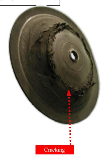
You will notice *bubbling*, *cracking or discoloration of the diaphragm* in which material of the diaphragm could be so bad it pulls away from it's internal lining. This situation can be avoided by reviewing the application to find a better material.
